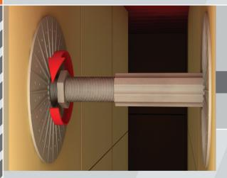
Void Gard® is in position and load is secured against lateral shifting.
